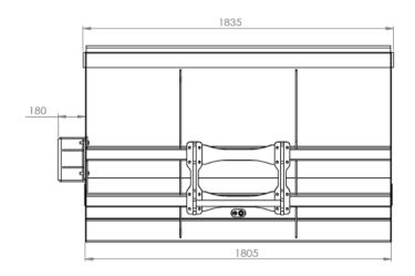
Loading capacity: **1,4 m<sup>3</sup>** Spreading wide: **5-6 m** Net weight: **500 kg** Gross weight: **550 kg** HS code: **84368090**
